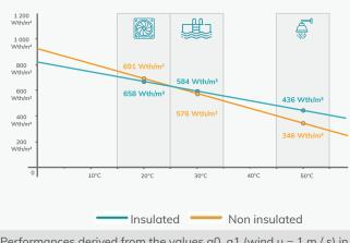
Performances derived from the values a0, a1 (wind u = 1 m / s) in STC conditions (T = 25  $^{\circ}$  C, G = 1000 W / m²)
